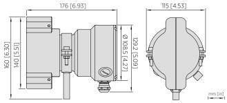
Dimensions PR53M tube fitting
